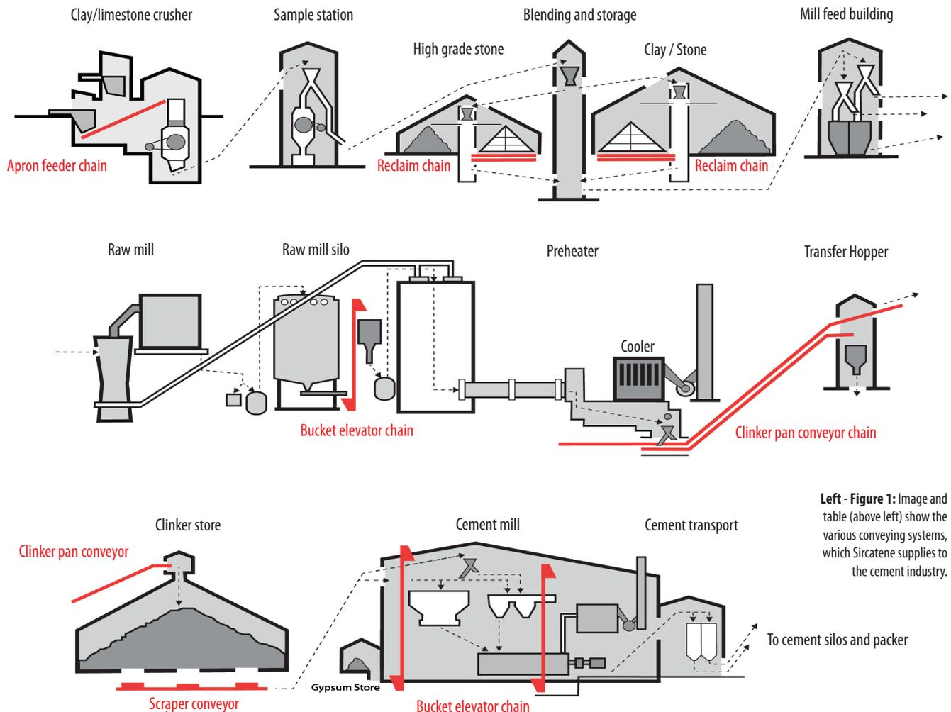
**Left - Figure 1:** Image and table (above left) show the various conveying systems, which Sircatene supplies to the cement industry.
